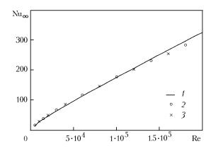
Fig. 2. Limiting local Nusselt number  $Nu_{\infty}$  vs. Reynolds number in air motion in a circular pipe: 1) calculation from (25); 2) (26); 3) (27).
