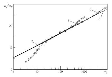
Fig. 1. Dimensionless velocity profiles  $u/u_*$  in the case of turbulent air flow in a circular pipe: 1 and 2) calculation from formulas (8); 3) logarithmic profile (9) for  $\kappa = 0.41$  and C = 5.5 (1) Re = 40,260; 2 and 3) 429,200); points, experimental results [4].
